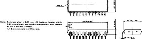
0.25 mm of their true longitudinal position with respect to No. 1 and No. 24 leads. All dimensions are in millimeters 2,54 ± 0.25 2.5 MIN. 0.5 ± 0.15 17.4 MAX
